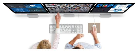
It is capable to manage several monitors with single keyboard and mouse set. By freely sliding the mouse cursor across monitors, the operator is able to manage any remote computers within the system.
