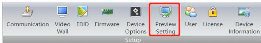
Enter desired IP address, subnet mask and gateway. Trigger “Display preview image on video wall”, you can preview input source and video wall display at software.
